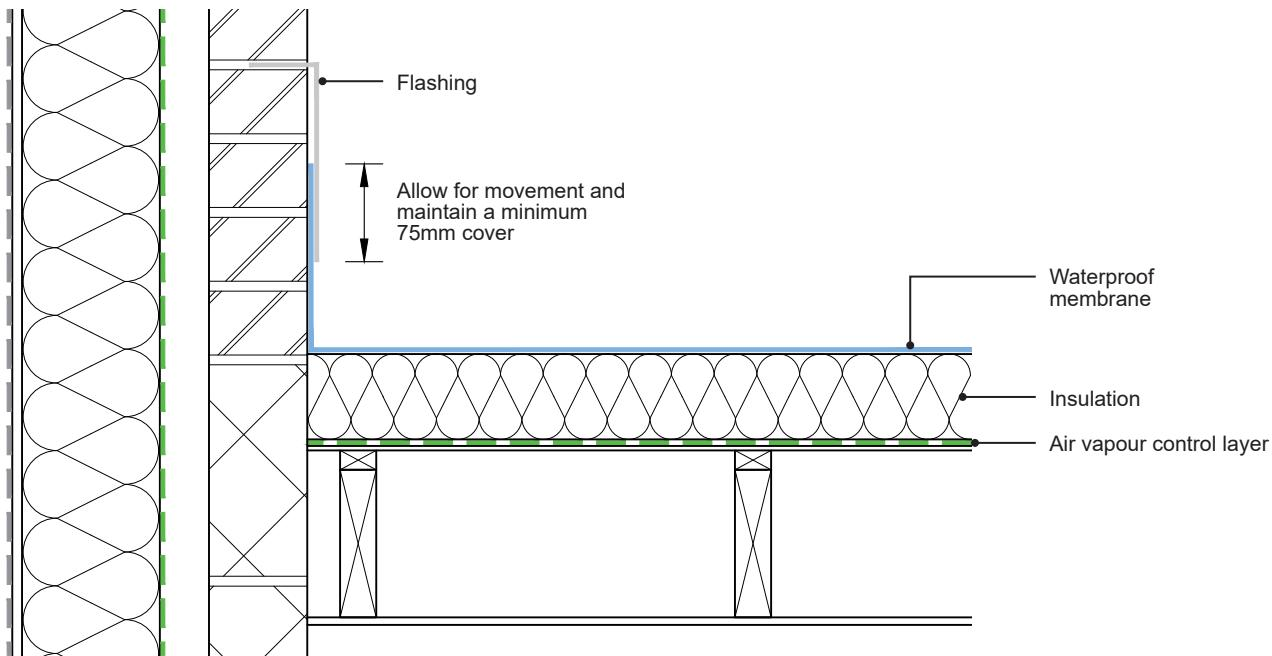
Where a timber frame structure abuts a masonry structure, allowance should be made to accommodate movement in the timber frame and ensure the appropriate cover is maintained.
