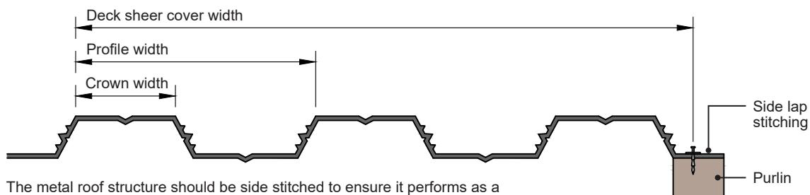
The metal roof structure should be side stitched to ensure it performs as a continuous plane layer (unless the manufacturer states otherwise).
