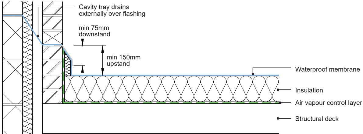
Insulation fully wrapped around by air vapour control layer and waterproof membrane.
